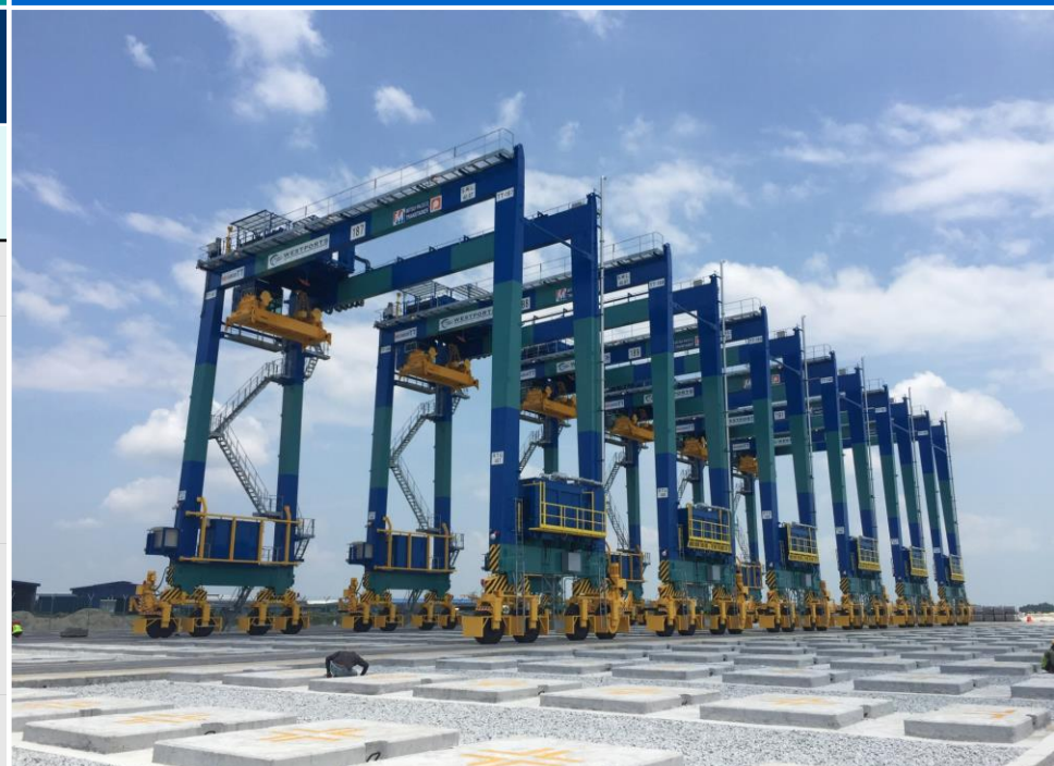
New Rubber Tyred Gantry cranes ready to be deployed at the recently completed container yard
