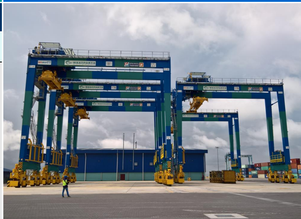
Newly delivered Rubber Tyred Gantry Cranes that are in the Testing & Commissioning Phase
